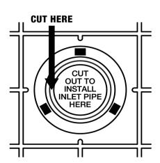
The three tabs at the base of the Inlet Pipe lock into the three holes in the top of the WaterUps cell. Apply some pressure to the Inlet Pipe as it is inserted until it clicks into the cell.
