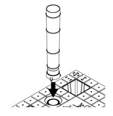
Take the WaterUps cell and Inlet assembly and place into the Reservoir base. Engage the tabs on each side to ensure Cell and Base stay together.
